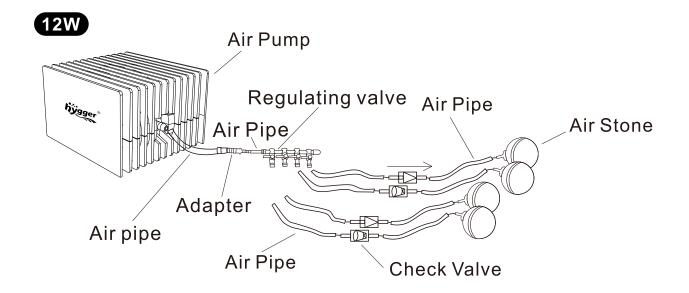
\*Reminder: This air pump does not include air stones. To ensure that the airflow is evenly distributed among each outlet, please use the same size of air stones or air diffusers.
